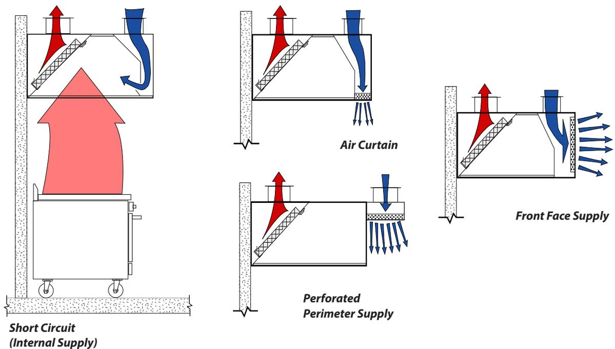
**Figure 1. Types of Makeup Air Supply Integrated with the Hood.**
