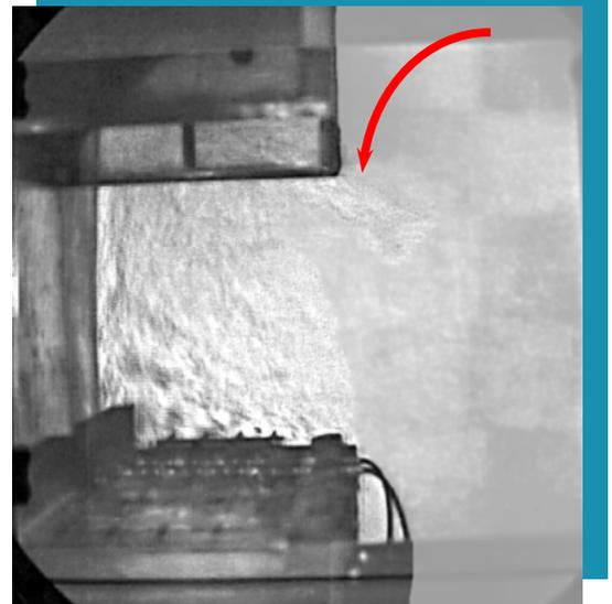
**Figure 6. Thermal Plume Pulled Outside Hood by the Air Discharged from a 4-Way Diffuser.**
